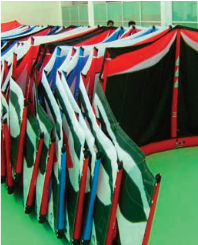
Kites receive an eight hour inflation test.
